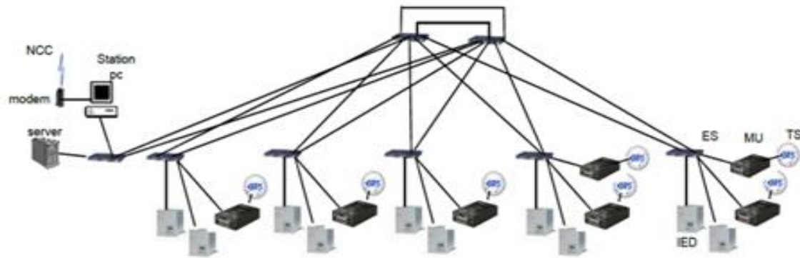
Figure 3 Star Ring Structure
